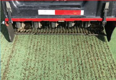
**Measuring a mere 7mm in diameter for the standard or 9mm for the XL.**
